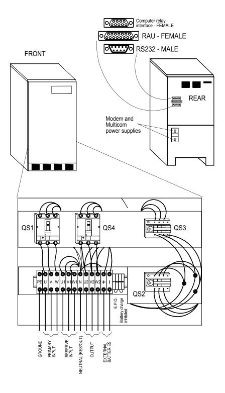
Figure 23 - 36 – 24/30/36kVA: Cable Connections
